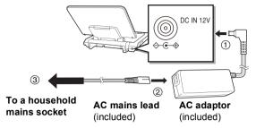
The unit is in the standby condition (the [む] indicator lights) when the AC mains lead is connected. The primary circuit is always "live" as long as the AC adaptor is connected to an electrical outlet.
