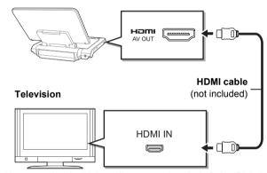
You can enjoy the high quality surround audio in Dolby Digital Plus, Dolby TrueHD, and DTS-HD by connecting this unit to the HDMI compatible multi-channel amplifier. (⇒ 34) (Only when connected to an amplifier compatible with each audio)
