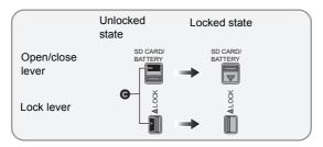
Lock securely to the points where the red portion of the open/close lever and LOCK lever are no longer visible.
