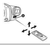
• The remote control is intended for indoor operation. Outdoors or under strong light, the unit may not operate properly even within the usable ranges.
