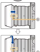
3 Rotate the lens hood in the direction of the arrow until it clicks into place, and align the stop position © on the lens hood with the index on the tip of the lens.
