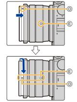
2 Rotate the decoration ring in the direction of the arrow to align the mounting position ① on the decoration ring with the lens fitting mark ⑤.
