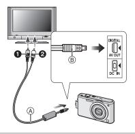
1 Connect the AV cable (A) (supplied) to the [AV OUT] socket on the camera.
