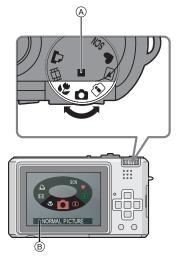
• The above screen (B) appears on the LCD monitor if the mode dial is rotated. (P20) The mode currently selected appears on the LCD monitor when the camera is turned on.
