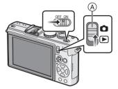
Switch the mode by rotating the mode dial.
