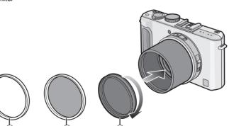
• Ensure that the screw parts of the lens adaptor and the filter are properly tightened.
