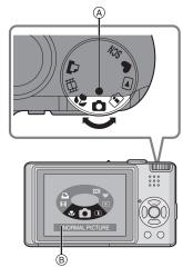
• The above screen (B) appears on the LCD monitor if the mode dial is rotated. (P18) The mode currently selected appears on the LCD monitor when the camera is turned on.
