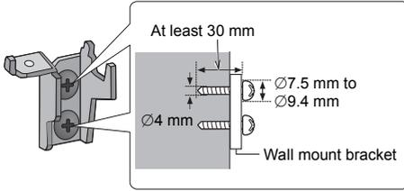
**3** Fix the safety holder onto the unit with the screw (supplied).
