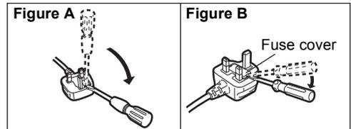
2. Replace the fuse and close or attach the fuse cover.
