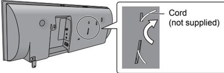
**5** Hook the unit securely onto the wall mount brackets with both hands.
