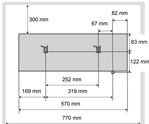
**2** Attach the wall mount bracket to the wall with 2 screws (not supplied). (Both sides)
