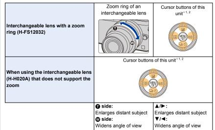
\*1 When operating the zoom with the cursor buttons, press the function button to which [Zoom Control] in [Fn Button Set] (P43) of the [Custom] menu has been set.
