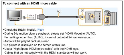
"High Speed HDMI micro cable" (Type D-Type A plug, up to 2 m (6.6 feet) long)
