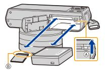
Pull the lever (A) in the direction of the arrow to remove the battery.
