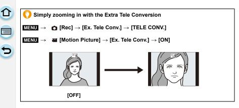
When the Extra Tele Conversion is used, angle of view for still pictures will be different from the angle of view for motion pictures because the zoom factor is different between them.
