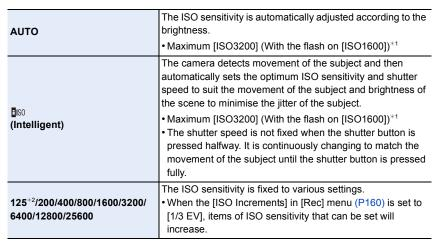
\*1 When the [ISO Limit Set] (P159) of [Rec] menu is set to anything except [OFF], it is set automatically within the value set in [ISO Limit Set].
