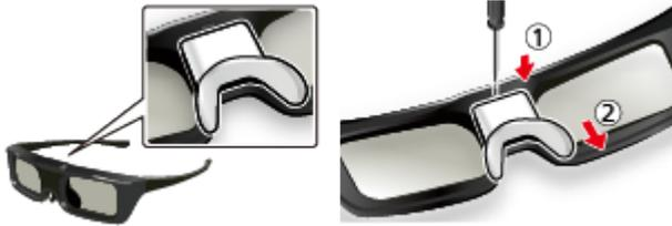
2. Replace the battery (coin-shaped lithium battery CR2025).
