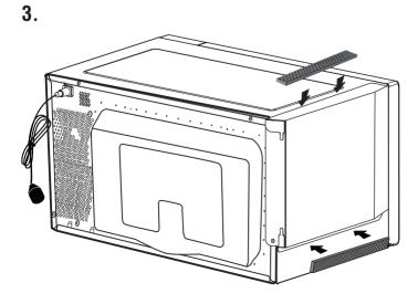
Put a piece of the tape on top of oven and left duct and put a piece of the tape on side of oven and left duct.
