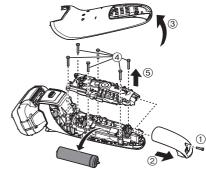
For environmental protection and recycling of materials This shaver contains a Lithium-ion battery.
