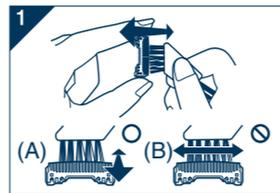
1. Clean the inner blades using the short brush by moving it in direction (A). Clean the system outer foil, the shaver body and the trimmer using the long brush.
