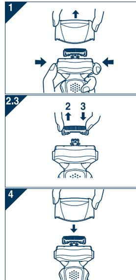
1. Press the system outer foil release buttons and lift the system outer foil upwards as illustrated.
