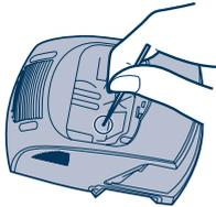
Beard trimmings may clog the drain at the bottom of the cleaning tray.
