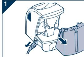
1. Be sure to remove the water tank and the appliance plug from the self-cleaning recharger.
