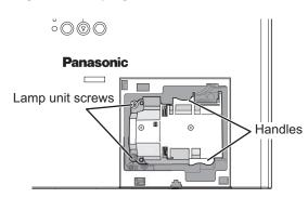
4 Press in the lamp unit until it clicks and make sure the unit is installed securely. Tighten the 2 lamp unit screws securely with a Phillipshead screwdriver.
