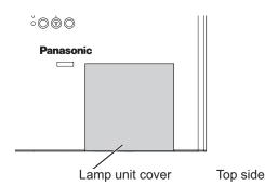
3 Use a Phillips-head screwdriver to loosen the 2 lamp unit screws. Pull the used lamp unit gently from the projector.
