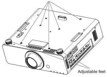
Screw holes for ceiling mount (M6)
