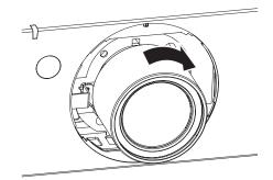
3) Attach the projection lens cover aligning the marking (groove \*1) with the tip of the arrow on the projector (\*2), and secure the projection lens cover by turning it until groove \*1 aligns with the \*3 ■ marking.
