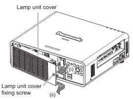
3) Use a Philips screwdriver to remove the lamp unit fixing screws (three screws each), and then holding the handles, pull out the lamp unit from the projector.
