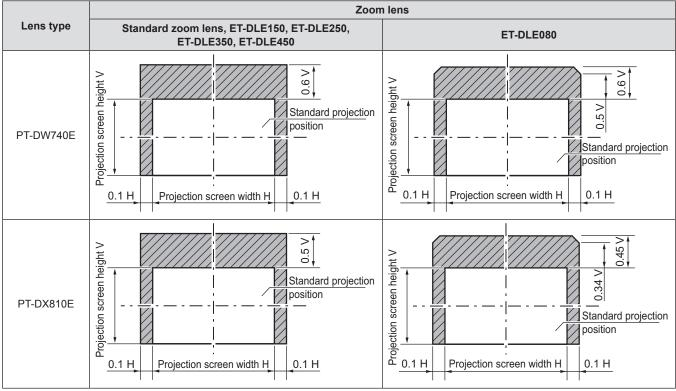
\* The numerical values in the diagrams above represent a case in which the projector is set on a desk/floor.
