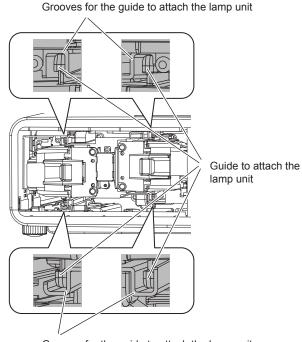
Grooves for the guide to attach the lamp unit
