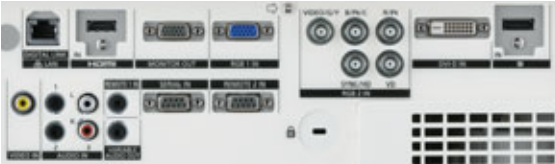
Terminal layout for PT-EZ580/EZ580L/EW640L/EW640L/EX610L/EX610L
