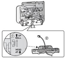
3 Insert the lower tabs of the adaptor into the unit's bottom slots (1), then insert by pushing
