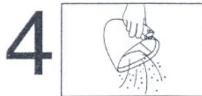
Remove the filter and empty dirt and dust.
