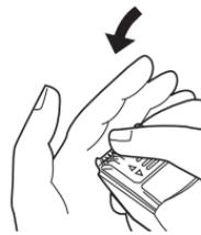
3. Brush off any hair trimmings from the main body and from around the blade.
