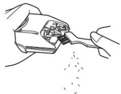
4. Brush any hair trimmings out from between the stationary blade and the moving blade while pressing down the cleaning lever to raise the moving blade.
