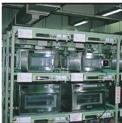
Endurance test at intermittent operation* 4 On (60s) and off (30s) 200.000 times; On (20s) and off (10s) 200.000 times
