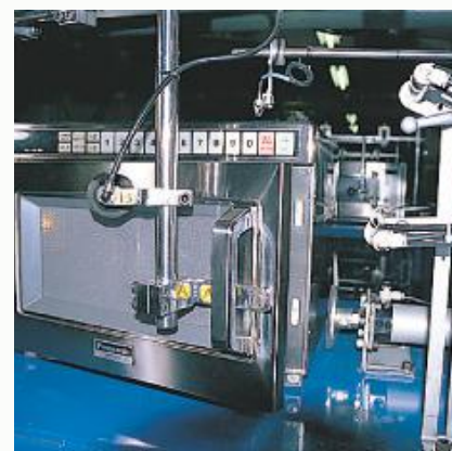
Endurance test of door (opening and closing)* 4 400.000x opening and closing the door
