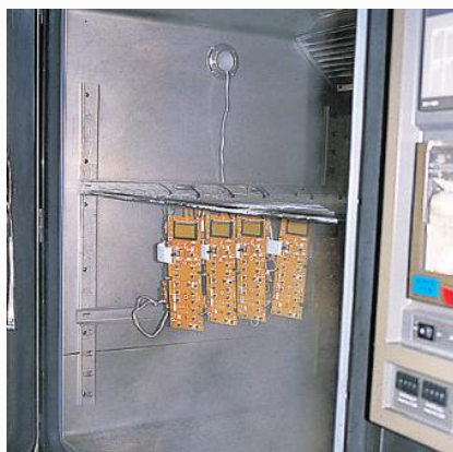
Circuit boards stress test* 4 Temperature of -40°C to +85°C, relative humidity 85 %
