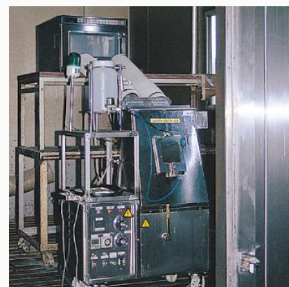
Dust and vapour test* 4 Operating in dust and vapour at a temperature of 40°C and a relative humidity of 95 %
