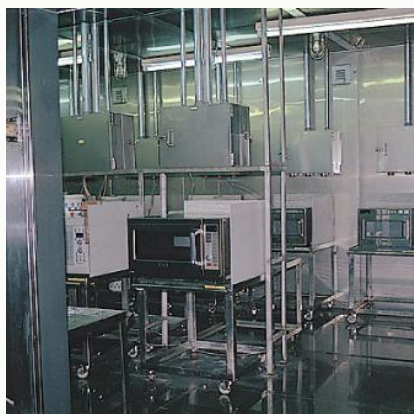
Combined stress test* 4 Temperature of 0°C to 40°C, relative humidity 85 %
