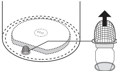
The filter can be removed by pulling firmly on it.
