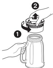
Turn blender container base counterclockwise to disassemble.
