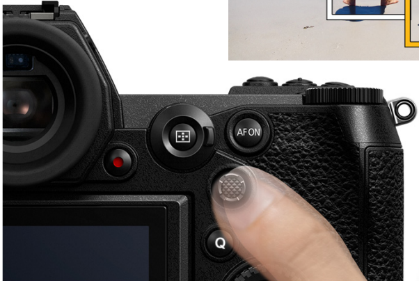
Pressing the joystick moves the main AF area toward the right.
