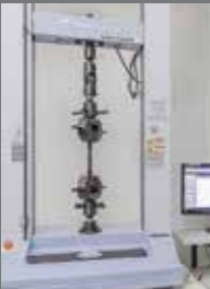
The strength of the resin material used in a propeller fan is confirmed by a tension test
