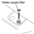
Remove the dust of water supply filter.
