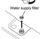
Remove the dust of water supply filter.
