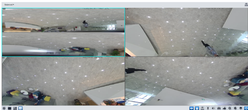
4PTZ view mode (you need to switch the stream mode in the fisheye parameter interface)
