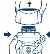
1. Press the foil frame release buttons and lift the outer foil section upwards as illustrated.
