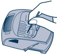
Beard trimmings may clog the drain at the bottom of the cleaning tray. In this case, you cannot clean or dry the shaver. Push the beard trimmings down through the drain with a tooth pick etc.
