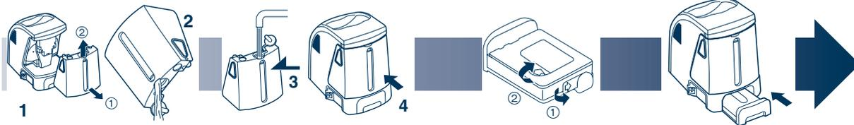
**1** Remove the water tank and then open the water tank cap.
