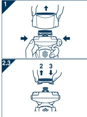
1. Press the foil frame release buttons and lift the outer foil section upwards as illustrated.
