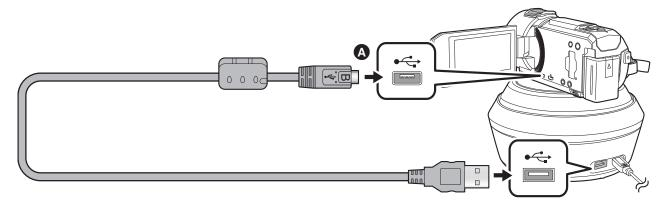
Turn the side with the symbol down to connect the micro B end of the USB Cable to the USB terminal of this unit.
