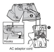
3 Insert the hooks on the wall mounting adaptor into holes **(A)** and **(B)** on the base unit.
