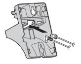
Tuck the telephone line cord inside the wall mounting adaptor (1). Connect the AC adaptor cord and telephone line cord (2).
