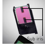
The sub iris cuts light leakage.
