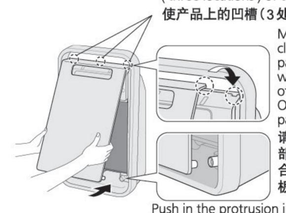
Make sure that the clutch of the front panel engages well with the indentations of the main unit. Otherwise the front panel may fall. 请将前面板的钩爪
