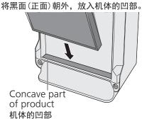
3 Toggle the filter hook downward, and secure filters.
