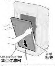
With the black side (front side) towards you and the label side up, fit it into the concave part of the main unit.
