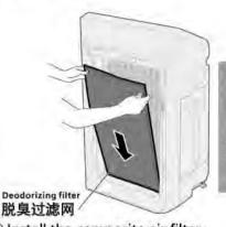
(2) Install the composite air filter. (There is distinction between the inside and outside, upper and
