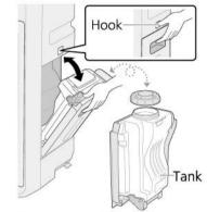
The upper position and lower position of the tank shall be reversed when you fill it with water to that when you install it back.
