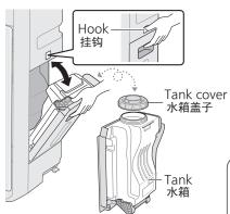
(2)Fill the tank with water. 水箱放入水
