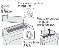
2 Slightly bend the middle of louver, and insert the other side into the other hole. 稍微弯曲导风板中部,将另一端插入圆形孔。
