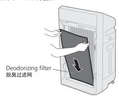
(2)Install the HEPA composite filter. (There is distinction between inside and outside, no distinction between upper and lower.)
