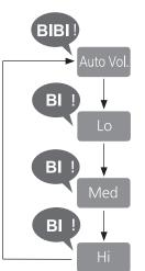
Automatically adjust the air volume according to the air pollution and humidity detected by sensor, and purify air or humidify by optimal air volume. 根据感应器检测的空气污染程度和湿度,自动调节风量,利用最佳的风量净化空气或加湿。
