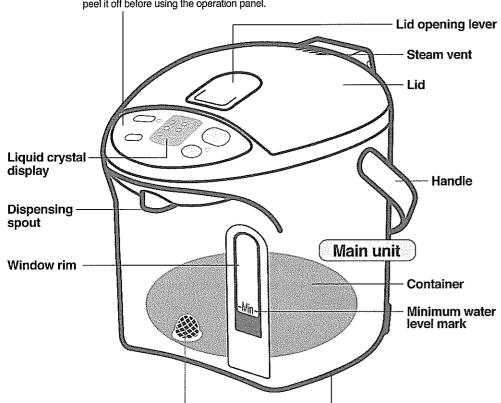
Rotating base (360 degrees) When rotating the pot, do not allow Mesh filter the cord to wind around the unit.
