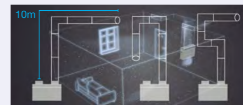
Bend once Bend twice Bend three times Based on in-house test result, even with a total ductwork length up to 10m, effectiveness of nanoe™ X is maintained.
