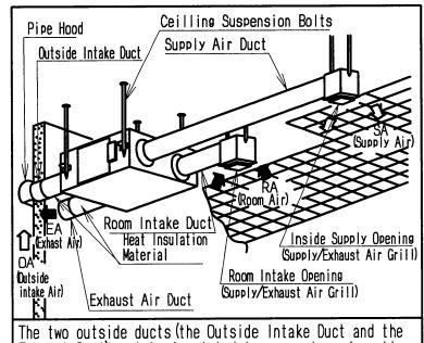
Exhaust Duct) must be insulated to prevent condensation (Material; Glass wool, Thickness; 25)
