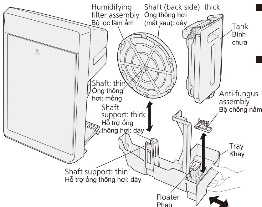
■ The humidifying filter assembly has thick shaft and thin shaft. Please be cautious when installing it back to tray.
