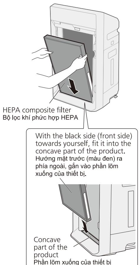
(3) Toggle the filter hook downward to secure the filter.
