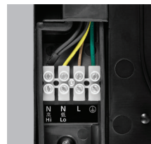
Power Supply Terminal
