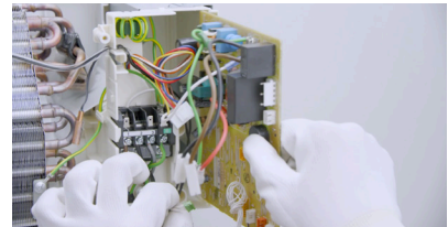
Pull out main PCB, Screw-free design makes it easy to remove PCB.
