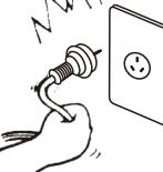
Unplugging roughly may damage the power cord and may cause electric shock, short circuit or fire.
