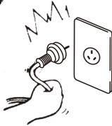
Unplugging roughly may damage the power cord and may cause electric shock, short circuit or fire.
