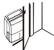
If there is insufficient ventilation, overheating and fire may occur.
