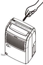
The rotating fan inside the unit could cause injury.
