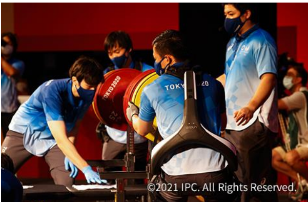
Image: "Power Assist Suits" that serve to lighten the physical burden placed on the staff as they lift weights
