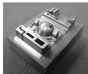
(a) By Hybrid system of metal powder bed fusion and milling
