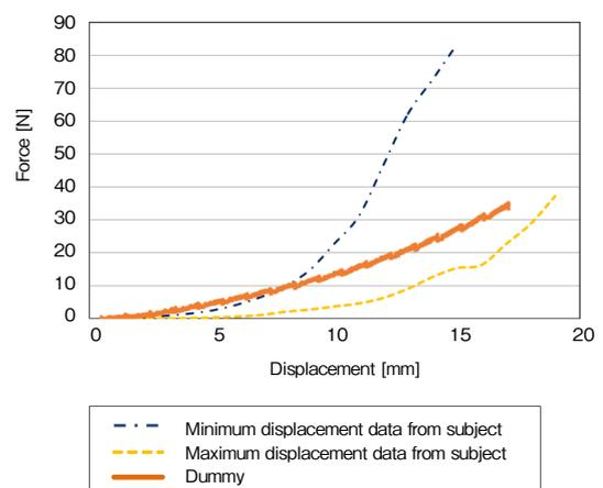
Fig. 7 Relationship between force [N] and displacement [mm] of maximum and minimum displacement data from 15 subjects and pain-sensing dummy at non-dominant forearm point
