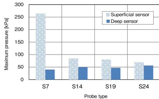
Fig. 9 Maximum pressure in superficial sensor and deep sensor during compression at pain-sensing dummy with 7 mm × 7 mm (S7), 14 mm × 14 mm (S14), 19 mm × 19 mm (S19), and 24 mm × 24 mm (S24) square probe at the same force with
