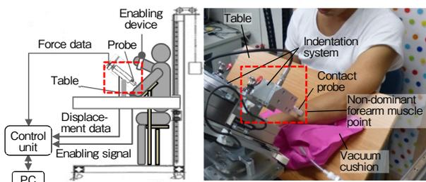
Fig. 5 Indentation system schematic (a), Indentation system at non-dominant forearm muscle point using S14 probe during the experiment (b)
