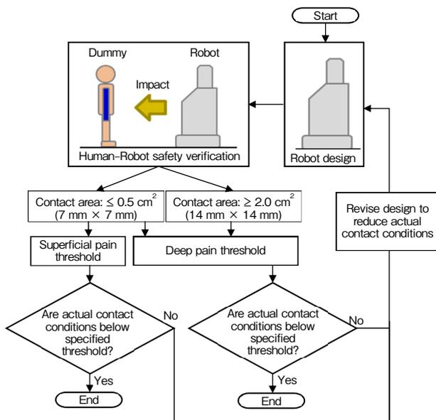
Fig. 10 Our hypothesis of the relationship between contact area and 2 types of pain (superficial and deep pain) according to the results from pain-sensing system with example of flowchart for application using pain threshold as a human-robot safety limit
