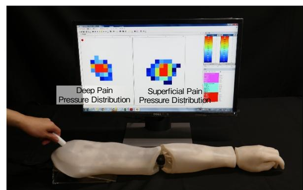
Fig. 6 Arm part of pain-sensing system showing pressure distribution at superficial layer sensor and deep layer sensor around deltoid muscle area
